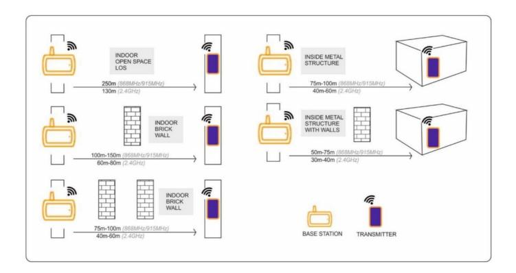
For large installations or with lots of internal wall or structures, routers can be added to expand the operating distance of the transmitters.
