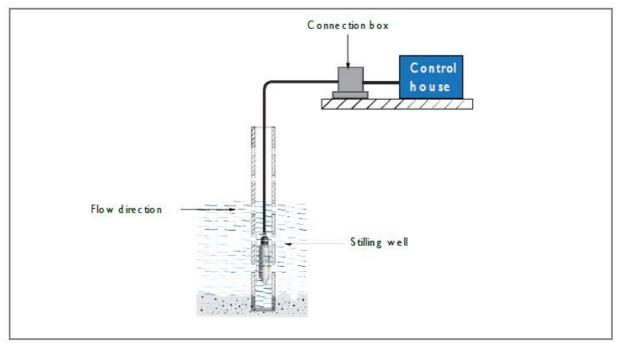
A stilling well is recommended when there is a flowing liquid. A stilling well will dampen disruptions and provide a steady level for an accurate measurement.
