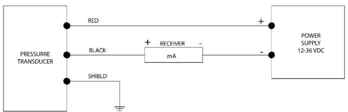
The maximum receiver load resistance (RLmax) for the DC power supply voltage (Vs) is expressed as:
