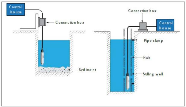
Place the transmitter away from liquid resource to avoid effects of vibration and pressure influence. A stilling well is recommended for the best results.
