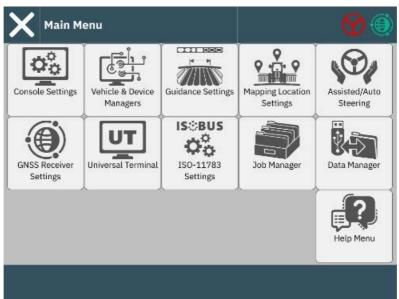
WARNING! If your system uses an ISOBUS device and the console is at v1.00/v1.01/v1.02, contact your local dealer or TeeJet Customer Service BEFORE updating your console. After updating a v1.00/v1.01/v1.02 console to v1.10 or above, an unlock code will be required to access the Universal Terminal (UT) feature.5
