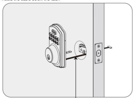
**IMPORTANT:** Bolt Must be in unlock Position note horizontal orientation of torque blade.
