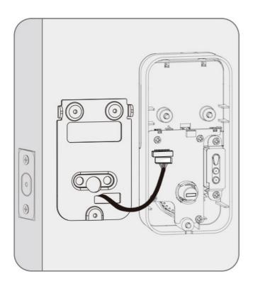
Rotate the Thumb turn in vertical Position and insert the horizontal orientation of torque blade into the interior assembly lock switch
