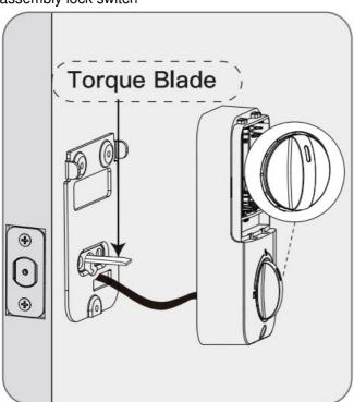
Secure the interior assembly with the Supplied Secure.
