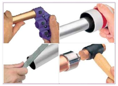
2. Remove any burrs or sharp edges from the external tube end using either the T110 (Tectite Classic and Tectite Pro) or the T115 (Tectite Sprint and Tectite Carbon) 3-in-1 Tectite deburring, scribe tool and socket depth marker, or the S120 deburring tool from the XPress accessories range. Also, ensure the internal bore is deburred. For deburring stainless steel tube ends a fine-toothed file should be used.
