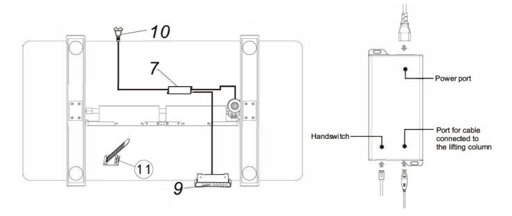
Use the cable tie(11) to fix all the connection cables on the desk to keep it clean.
