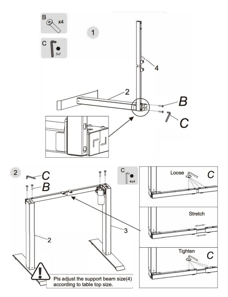
Lay Column(2) down, just like picture 1 shows, then install (4), use wrench(C) to tighten the screws(B). Install Column(3) just as picture 2 shows.
