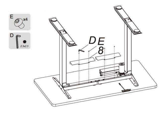
Install(8), use 2.5\*2.5 wrench(D) to tighten the screws(E).
