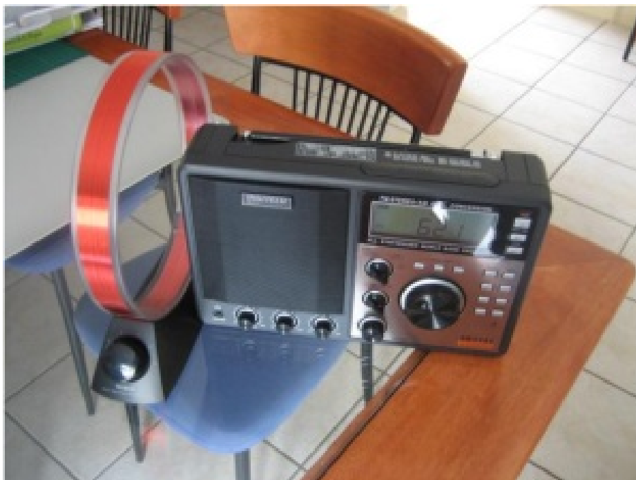
Jaycar AR-1747 AM/FM Shortwave radio with the Loop in action
