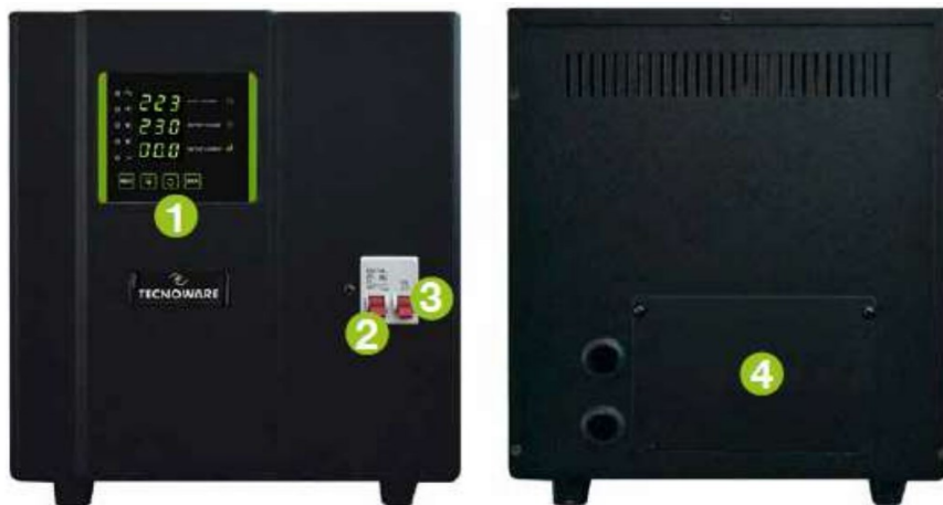
Figure 4 – Front and Rear side FSTESM4K5M, FSTESM7K5M and FSTESM10KM (1. Display, 2. Stabilizer Breaker, 3. Bypass Breaker, 4. Terminal Block Access Panel)
