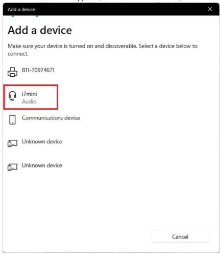
Thus, the system will automatically connect to that device; (If a pairing code is needed, please enter it based on the prompts.) When connected, click [Completed] to finish.
