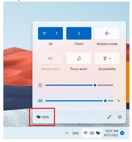
Click the battery level icon in the pop-up menu to enter the settings page of power and battery management; [Balance: balance between system response and power consumption; best energy efficiency: prefer power saving, slower system response; best performance: prefer performance, reduced battery life with increased heat;]. (This function is not available for some models.)
