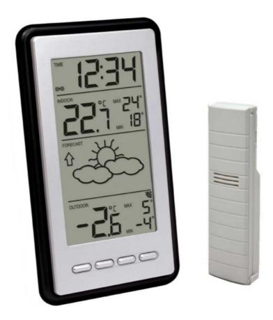
The WS9130 is a very popular wireless weather forecast station, featuring a weather trend indicator based on the air pressure change, plus indoor and outdoor temperature (via a remote sensor) and max/min records. The time is radio-controlled for accuracy, so you should never need to adjust it.
