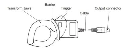
Barrier: It is a part providing protection against electrical shock and ensuring the minimum required air and creepage distances.
