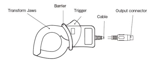
**Barrier**: It is a part providing protection against electrical shock and ensures the minimum required air and creepage distances.
