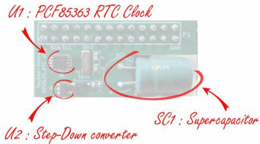
FIG 3 – PiRTC Main Components
