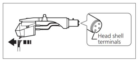
Wipe the headshell terminals occasionally. Wipe the headshell terminals with a soft cloth and fit the headshell to the tonearm.
