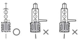
Tighten the screw for a cartridge.
