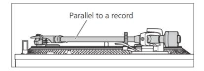
Return the tone arm to the armrest, clamp it with the arm clamp, and while pressing the arm lift down with your finger, turn the screw to adjust the height.
