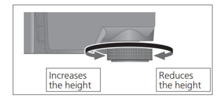
Raise the main unit to turn the insulators and adjust the height.
