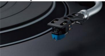
The SL-100C comes preinstalled with an Audio-Technica AT-VM95C cartridge, so you can listen to your favourite tunes in high fidelity right away. The tone arm height can be easily adjusted within a range of 6 mm, enabling the use of various other phono cartridges.
