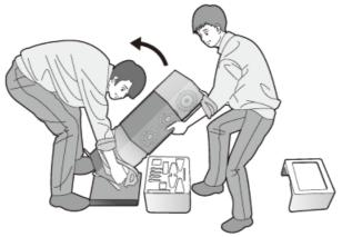
Remove the protective bags (2 pcs) and the cardboard covering the speaker. Hold the speaker so that it is tilted forward and move it to the installation location.
