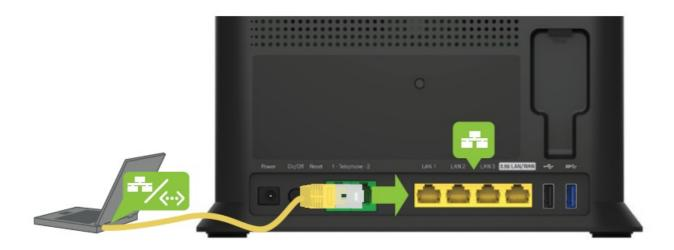
If you want to connect a device using a wired (Ethernet) connection:
