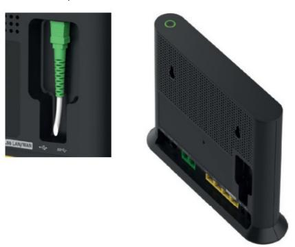
2. Take the other end of the fibre cable, remove the protective cap from the connector and then insert the connector in the optical termination point.
