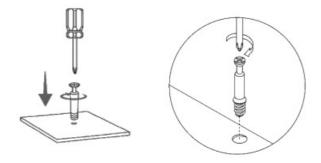
2. Place the other panel over the panel with the bolt, then insert the cam lock to join the bolt's head. If the cam lock does not want to enter, check its proper alignment. There might be a very small gap between the panels which is normal.
