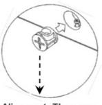
Alignment: The cross points towards the panel with the bolt.
