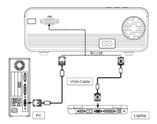
**NOTE:** The device and connection of the laptop may not be able to display images at the same time, if that happens, set the computer display attributes, and select CRT output mode.
