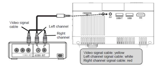
**Audio output:** Audio signal from the output port of the device, if you want to high-power play music input end connected to an external power amplifier.
