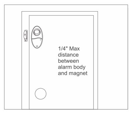
The magnet must be mounted no further than 1/4" from the alarm body – If the unit goes off continuously when you turn it on, check the distance between the magnet and alarm body. The magnetic sensor must be mounted on the left side of the alarm body. Be sure the arrow on the magnet lines up with the line on the left side of the alarm body.
