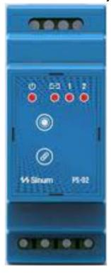
The PS-02m module is an electronic device equipped with 2 independent voltage-free relays enabling the user to control 2 independent devices. It is designed to be mounted on a DIN rail. It communicates with the Sinum central device by wire.
