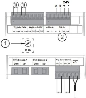
The KW-10m input / output card is a device that takes a part in the exchange of information between sensors and devices connected to the card and the Sinum Central device. KW-10m is equipped with:
