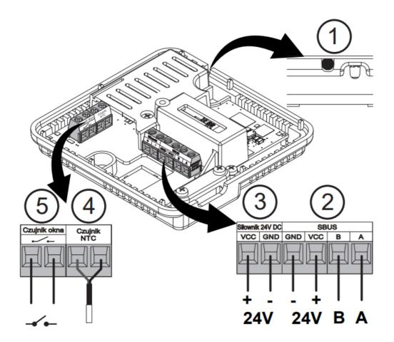
The KW-03m input card is a device that takes a part in the exchange of information between sensors and devices connected to the card and the Sinum Central device. KW-03m has a built-in temperature sensor. Communication with the Sinum central device is done by wire.
