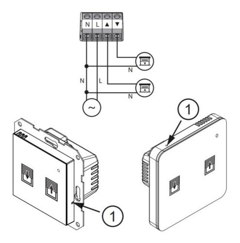
The FZ-02 / WZ-02 roller shutter switch is a device for controlling roller shutters with the use of the switch or the Sinum central device. Sinum allows the user to program specific conditions for raising / lowering the roller shutters. Communication with the Sinum central device is wireless. The FZ-02 / WZ-02 switch has a built-in light sensor which is used to adjust the button backlight brightness to ambient light level.
