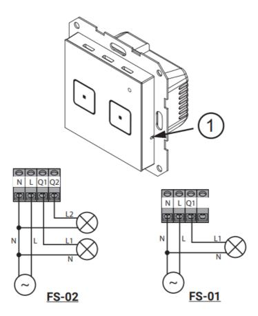
The FS-01 / FS-02 light switch is a device which enables you to control the light directly from the switch or with the use of a Signum central device, where the user may program the light to switch on and off in certain conditions. The switch communicates with the Signum central device wirelessly and the whole system allows the user to control the smart home with the use of mobile devices.
