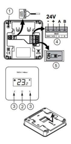
The R-S2 room regulator is equipped with a temperature and air humidity sensor.
