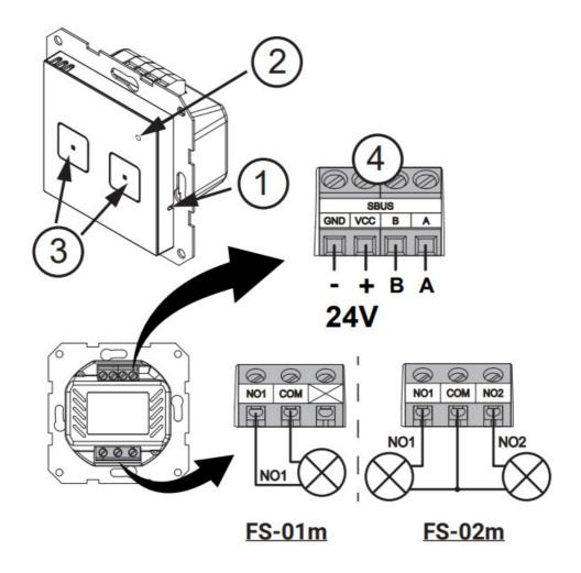
The FS-01m / FS-02m light switch is a device which enables you to control the light directly from the switch or with the use of a Signum central device, where the user may program the light to switch on and off in certain conditions. The switch communicates with the Signum Central device by wire and the whole system allows the user to control the smart home with the use of mobile devices.
