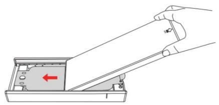
8. Peel off the secondary mask film and remove the phone from the application Box. The screen protecto should now be fully applied.
