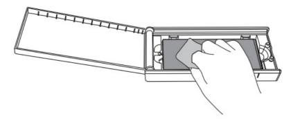
3. Peel off the mask film from the screen protector with the Step 1 label.
