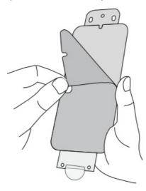
4. Secure the screen protector to the top of application box by placing the large plastic peg through the center hole of the top tab (this may come pre-installed), and inserting it into the indentation in the application box. Make sure the screen protector does not adhere to phone screen at this step.
