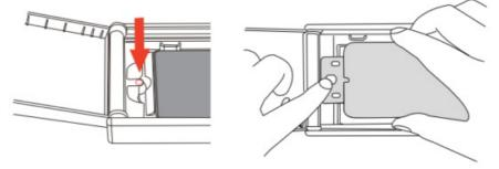
5. Align the holes in the tab on the bottom of the screen protector to the plastic pegs on the application box. This will help keep the protector in place. Make sure the screen protector does not adhere to phone screen at this step.
