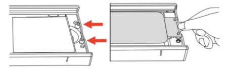
6. PULL the cover of the case over the device and it will roll along the tracks on the sides. This will help to apply the protector to the phone's screen. Pull all the way to the edge of the application case.
