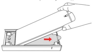
7. PUSH the cover of the case back over the phone the opposite way to help reinforce the protector's adhesion to the screen.
