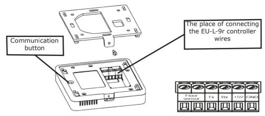
Mount the EU-R-9b sensor hanger on the wall and next fit the cover.
