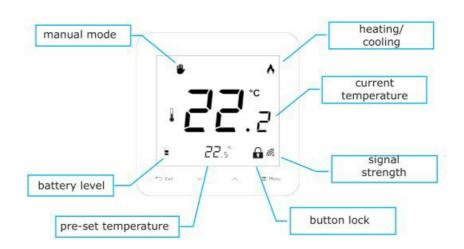
• Manual mode – the pre-set temperature may be adjusted manually in the main screen view using the buttons
