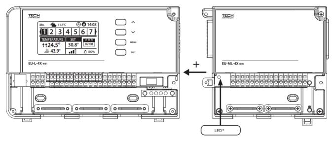
\*The LED lights up after connection to the main controller, regardless of whether the module is attached to a supply of power.
