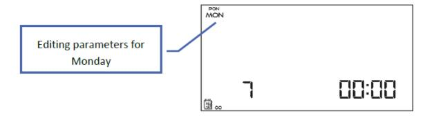
STEP 3 – ASSIGN COMFORT TEMPERATURE OR ECONOMICAL TEMPERATURE TO PARTICULAR HOURS An hour which is being edited is displayed on the controller screen. In order to assign comfort temperature, press
