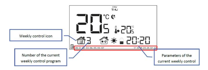
\* The display shows the hours when the comfort temperature applies. In the remaining time period economical temperature applies.
