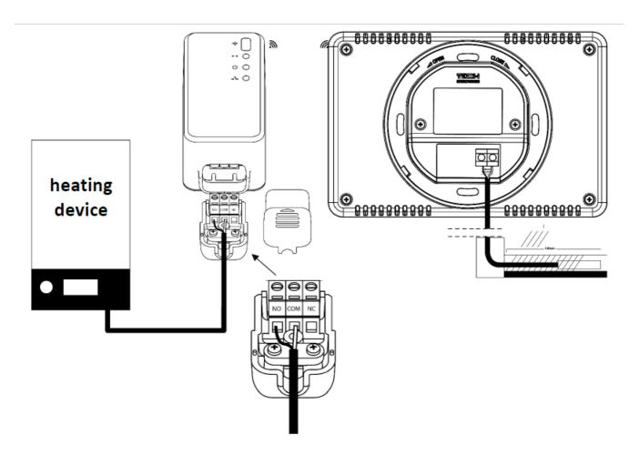
The EU-293v2 room regulator may be used as a wall-mountable panel. In order to mount it, place the rear part of the controller in the mounting box on the wall, insert the regulator and turn it slightly.
