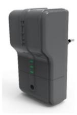
2. v2 module – it transmits the 'ON/OFF' signal from the v1 module to the main controller or the heating device.
