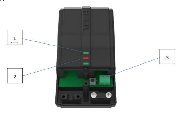
1. Room regulator status (control light ON – heating). It also signalises communication channel change as
