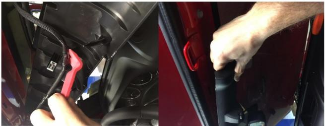
2. Continue running the SP-8100 wiring harness from the engine bay area to the area above the h rear view mirror at the TTO Switch Housing
