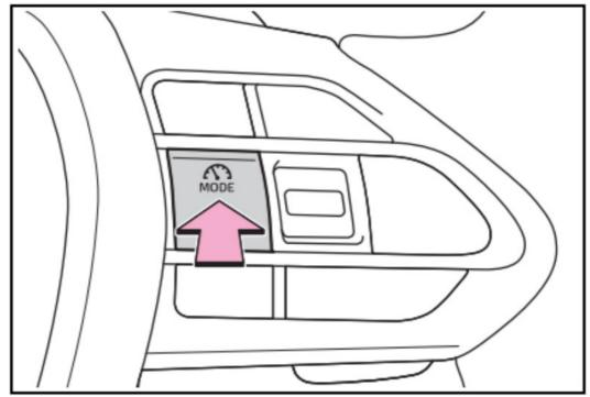
Using the accelerator pedal, accelerate or decelerate to the desired vehicle speed (approximately 30 km/h [20 mph] or more), and press the driving assist switch to set the set vehicle speed.
