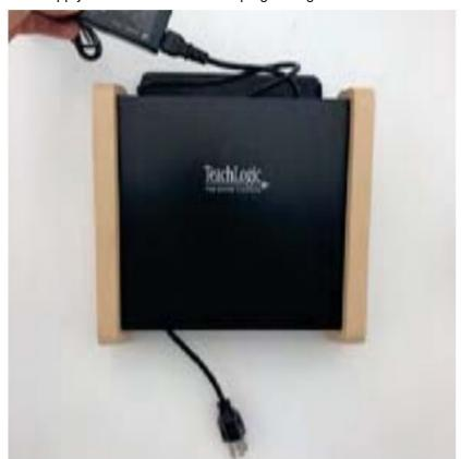
5. Place power supply in holding slot inside of cabinet.
