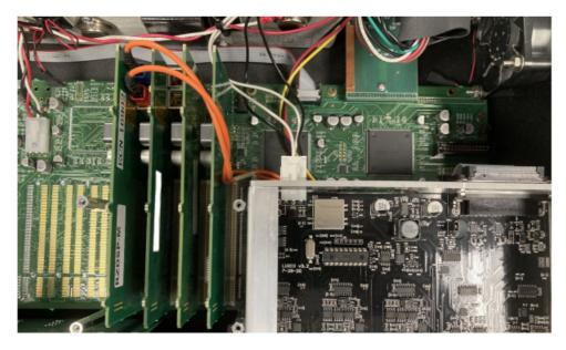
6. Reinstall the DSP plate and four screws with star washers that you removed in step #3, and put the lid back on the RZ10X. Your iCon (or other device supported by a RZDSP-M card) can now be connected to the RZ10X front panel.
