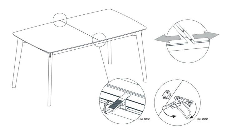
Take out extension leaves. Place the extension leaves and move the two halves of the top frame towards the extension leaves. Use the lock mechanism to x the top frame in place. If you prefer, you can use one extension
