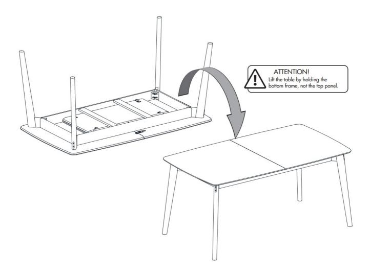
Release both lock mechanisms under the top panel and slide apart the two halves of the table top.
