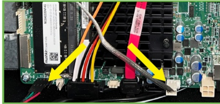
Closeup of LED power/reset and fan connections (board style 2)
