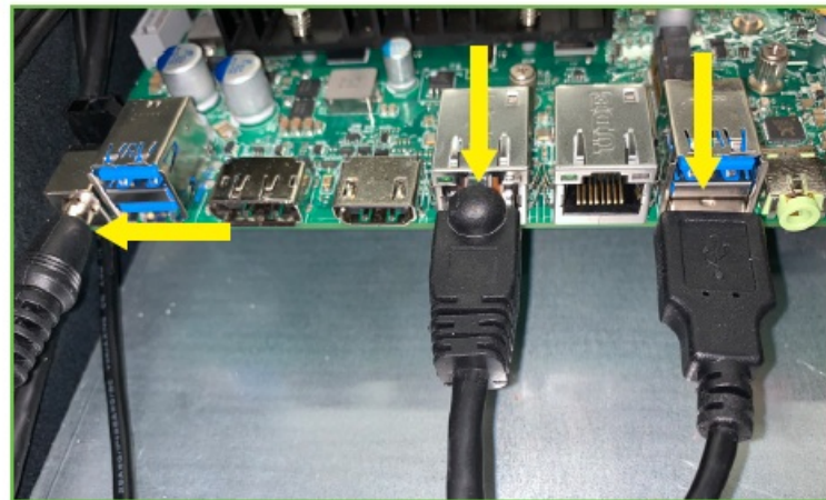
Closeup of Mother Board Power, Cloud Ethernet, and USB connections
