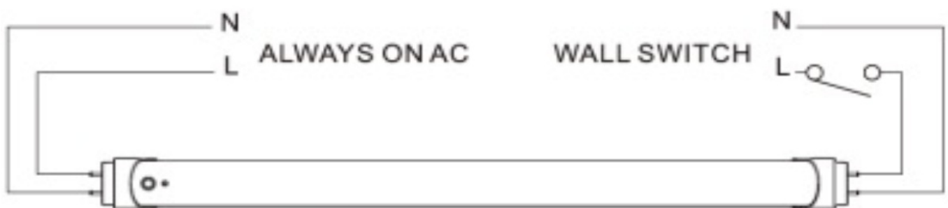
EMERGE LED tube wiring schematic
