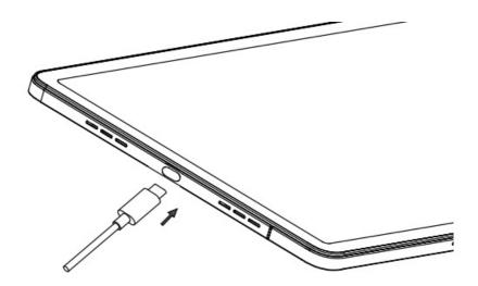
1. Your new tablet is partially charged. Charge the battery by using the USB-C cable and charger provided.
