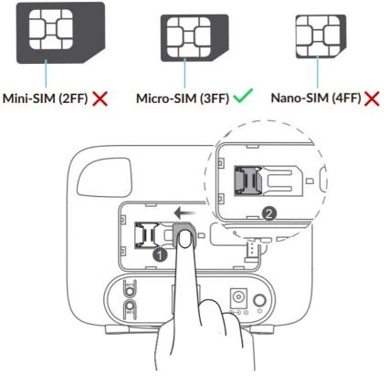
Be aware of the orientation of the SIM card. If the SIM card is inserted incorrectly, it may get jammed. Do not remove the micro SIM card when your device is in use.
