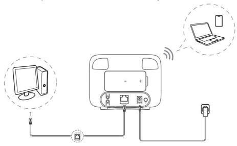
If your wireless device is WPS-enabled, you can also access the CPE Wi-Fi network through a WPS connection. Select one of the following options to make a WPS connection.
