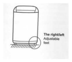
Lid and machine clearance: The machine must be at least 5 cm of free space clearance around itself.
