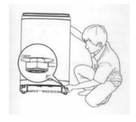
**IMPORTANT:** Adjustable feet are assembled on the left or right side depending on the different models.
