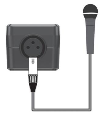
5. Move the Power switch to the ON position. If you have connected a condenser microphone, selec t the +48V position to supply phantom power. The 48V LED on the front panel will light red.
