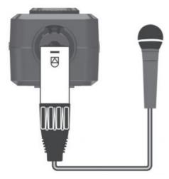
4. To enable phantom power move the 48 V power switch to the ON position. The 48 V LED on the front panel will light blue.
