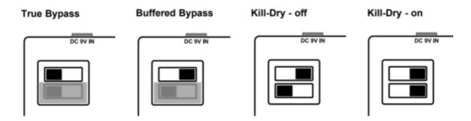
**True Bypass** – is a hard-wire bypass that gives absolutely no coloration of tone when the pedal is bypassed. Using True Bypass on all pedals is a perfect choice in setups with a few pedals and relatively short cables before and after the pedals.
