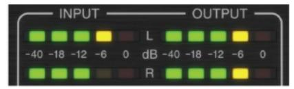
The meter section gives feedback about the incoming and outgoing audio signals. The input level displays the audio as it enters the plug-in, and is not affected by adjustments to the input level control or any other parameter. The output meter is affected by the results of the effect as well as the output level control parameter.
