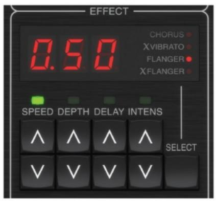
Press the SELECT button to rotate through the 4 effect styles. The red dot will indicate the current selection. Adjust the SPEED, DEPTH, DELAY and INTENSITY with the associate arrow buttons.
