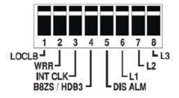
The DIP switch functions on the TC8619 are described below. To activate the function, set the appropriate switch to the On (Down) position.
