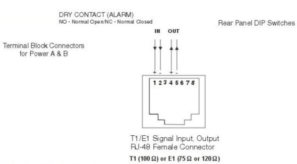
Note 1: The T1/E1 signal use the same pin connections on the RJ-48 female connector.
