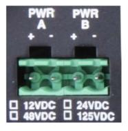
**Important** Read and only connect a supply voltage that corresponds to the type plate of your device. Make sure that the contact load capacity of the signal contact is not exceeded.
