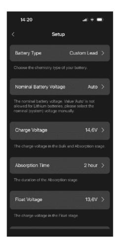
You will also notice that when Custom Lithium is selected, there are a lot less parameters to edit since a float stage and equalization are not possible for Lithium, as well as temperature compensation of the charge voltage. When you do wish to have a float stage for your lithium battery, please see chapter 3.2.1.
