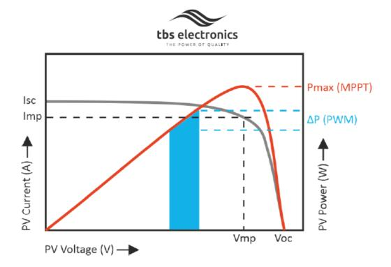
The blue area in the above graph ( $\Delta P$ ) represents the typical operating area of a traditional PWM type solar charge controller. As you can see, Pmax (MPPT) is higher than  $\Delta P$  (PWM).
