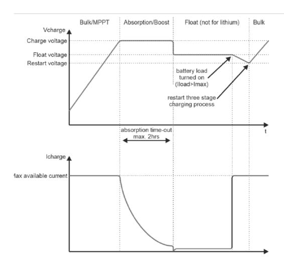
In the Bulk/MPPT stage the charger delivers full available output current and typically returns approximately 80% of charge back into the battery, once the charge voltage is reached. During this stage the charger runs in MPPT mode, transferring maximum PV power into the battery.
