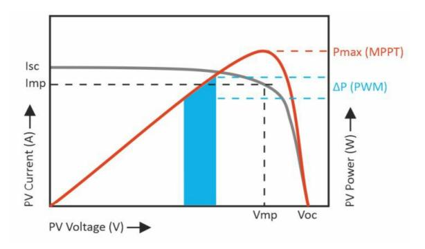
The blue area in the above graph ( $\Delta P$ ) represents the typical operating area of a traditional PWM type solar charge controller. As you can see, Pmax (MPPT) is higher than  $\Delta P$  (PWM).
