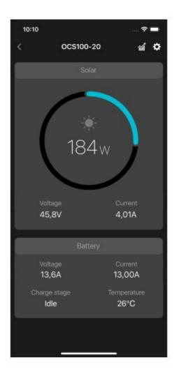
In main screen of the device you can observe all available real time data of the solar panels, the battery and the charging status. Once the sun icon is shown inside the solar power gauge, the charger is active. When the moon and stars icon is shown, the charger is inactive due to a lack of solar light.
