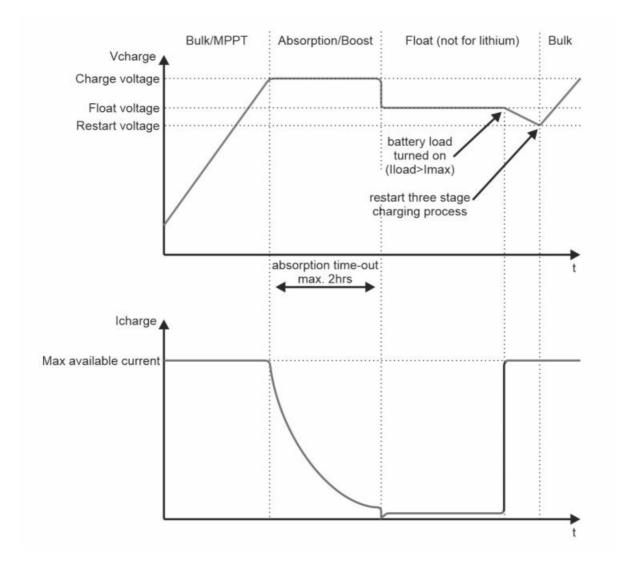
In the Bulk/MPPT stage the charger delivers full available output current and typically returns approximately 80% of charge back into the battery, once the charge voltage is reached. During this stage the charger runs in MPPT mode, transferring maximum PV power into the battery.
