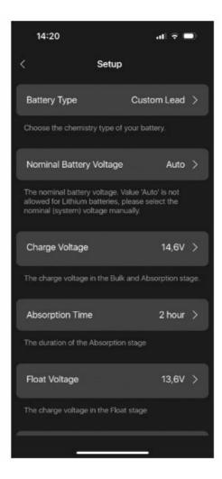
If any of the standard selectable battery types does not fulfil your requirements, there is a possibility to create your own battery type or charge program.
