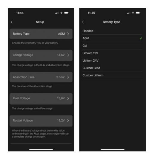
If from the settings screen you have pressed the Setup button, the first screen on the right will appear. In this screen you can select the desired battery type by pressing the upper button.
