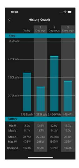
The history graph screen shows you the solar energy yield of the current day and previous days. Additionally it also indicates the minimum and maximum battery voltages, maximum charge current and charge power and total Amphours charged of each day. You can swipe left to show more days or rotate your device to enter landscape view.
